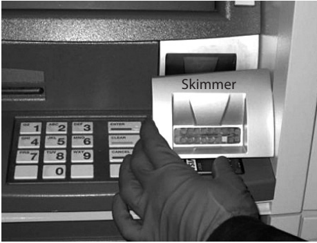
FIGURE 1 – Example of an ATM Skimmer
